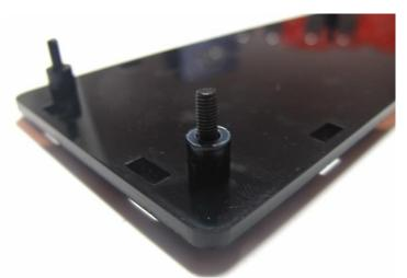
3. Put a clock printed circuit board on the screws and screw with 8mm spacers. Do not tighten the screws strongly because the plastic casing can crack.
