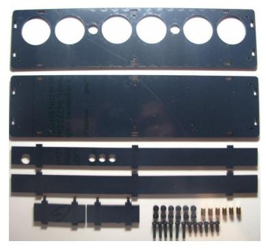
2. Insert six screws (3x16 mm) in plate holes and put a plastic 3mm spacers (2pcs) on each screw.
