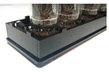
5. Cover the top lid and screw it by 10 mm screws. Do not tighten the screws strongly because the plastic lid can crack.
