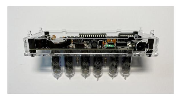
5. Cover the bottom lid and screw it by 6 mm screws. Do not tighten the screws strongly because the plastic lid can crack.
