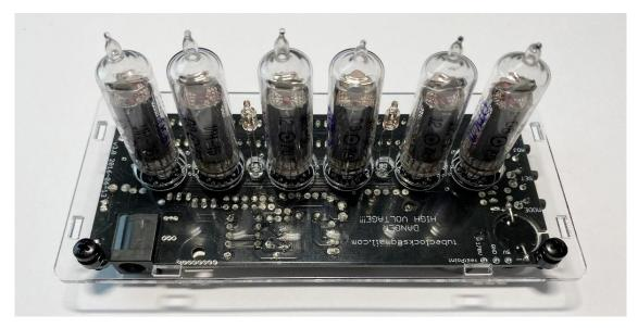
3. Screw spacers (10mm). Do not tighten the screws strongly because the plastic casing can crack.
