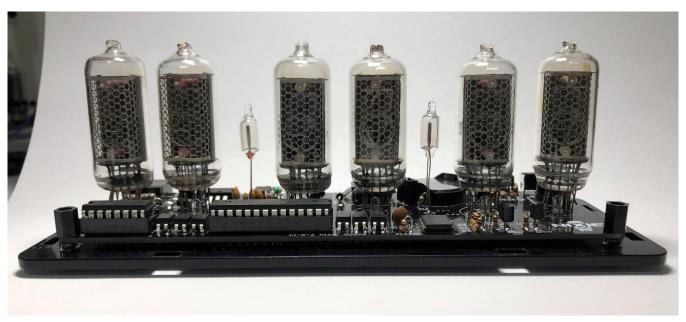
6. Fit plastic sides. Cover the top lid and screw it by 8 mm screws. Do not tighten the screws strongly because the plastic lid can crack.
