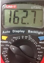
4.4. Test low voltage (LV) source operability. Touch the black probe on the GND test point and the red probe on the 5V test point. The voltage should measure between 4.8 and 5.2 Volts. If not, disconnect power and check all relevant joints quality and polarity.
