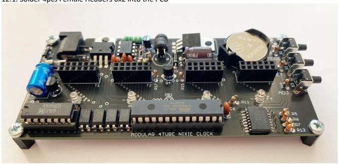
12.2. Solder 4pcs Male Headers 6x2 into the Cell PCB (Socket Side).
