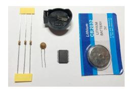
NOTE: An integrated circuit U5 DS3231 is in SMD (surface mount device) case, which is very difficult for soldering. Due to it soldered in advance.
