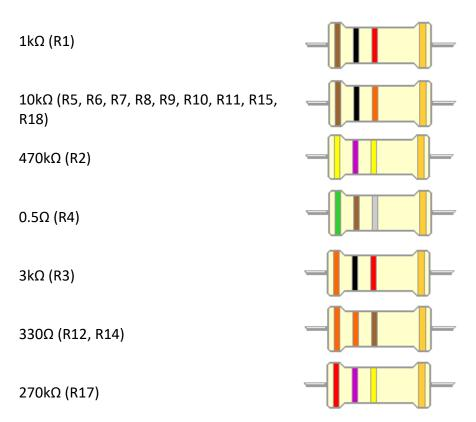
The resistors used in the kit are marked with four coloured bands to identify the value. Bands 1 and 2 identify the first two digits, band 3 is the Multiplier and band 4 is the tolerance.
