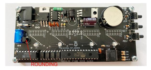
10.3. Plug in the power supply, and then check or all of the LEDs light up. If not, check all relevant joints quality and polarity. Do not continue with the assembly until the error will be corrected.
