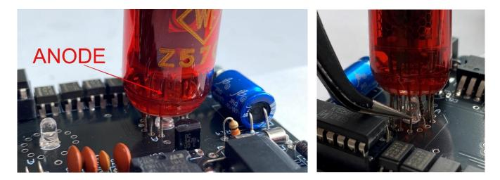
12.3. Install all tubes on the same height. Level tubes that they stand straight. After inserting a tube leads into the board, solder its two opposite leads first. This will hold the tube in place. Look at it carefully to check it proper height and reciprocal arrangement. It is important that tubes will not inclined to the sides. If not, it is easy to heat one or both leads and adjust the relevant tube. Only if everythis correct, solder the rest leads from opposite PCB side.
