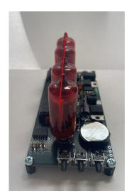
12.4. Solder Neon bulb DB1 in place on the PCB.
