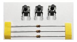
8.1. Parts S1-S3 are right-angle tactile button switches. Insert them into locations S1, S2 and S3, and make sure that they sit flat on the board. Solder all four pins of each switch.
